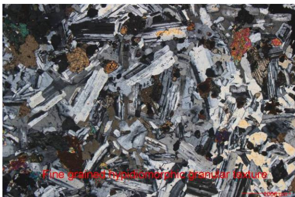
Fine grained hypidiomorphic granular texture (Crossed polarizers)
