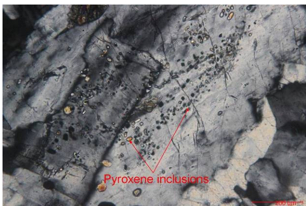
Pyroxene inclusions in plagioclase (Crossed polarizers)
