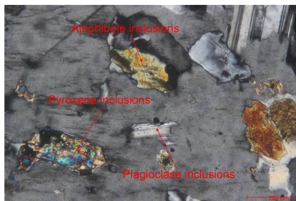
Plagioclase inclusions, pyroxene inclusions and amphibole inclusions in potash feldspar (Crossed polarizers)
